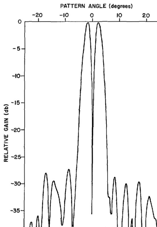
Fig. 7. Difference pattern of experimental array and modified "center-fed" ladder network.
