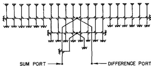
Fig. 4. Experimental array and modified "center-fed" ladder network.
