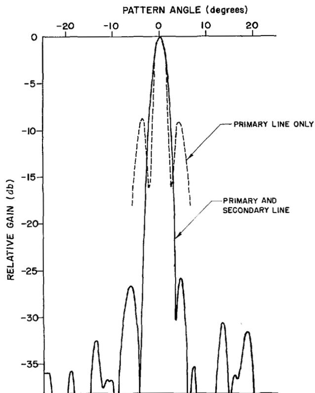
Fig. 6. Sum pattern of experimental array and modified "center-fed" ladder network.
