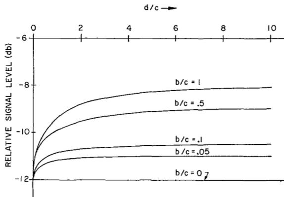
Fig. 3. Total signal along shadow boundary relative to signal at same observation point when both edges are removed.
