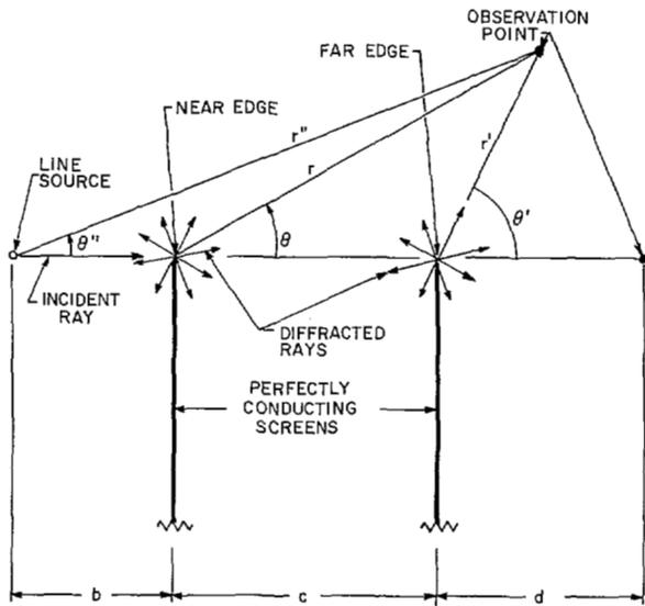
Fig. 1. Double knife-edge geometry.
