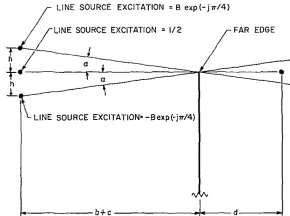
Fig. 2. Virtual sources providing proper incident field on far edge
