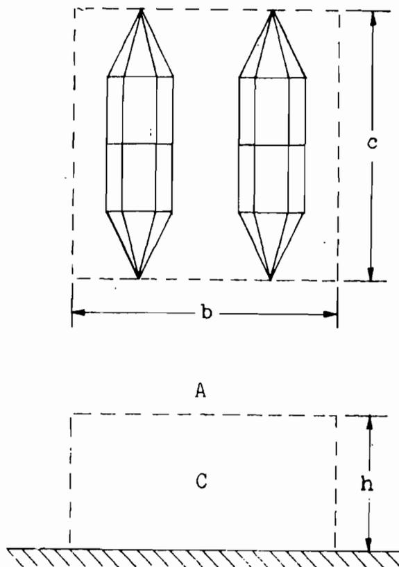
Fig. 1—Essential dimensions of flat-top antenna.
