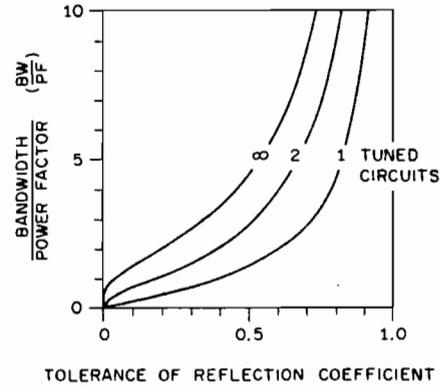
Fig. 3. Bandwidth of matching with tuned circuits.
