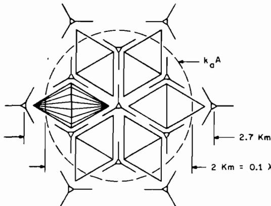
Fig. 17. Large VLF antenna (plan view).
