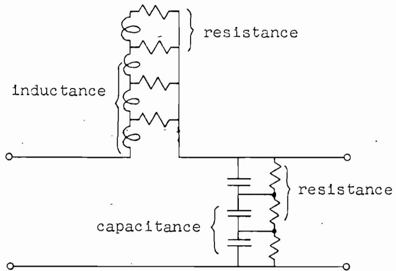
Fig. 4 - Transmission-line analog of space between ground and ionosphere.
