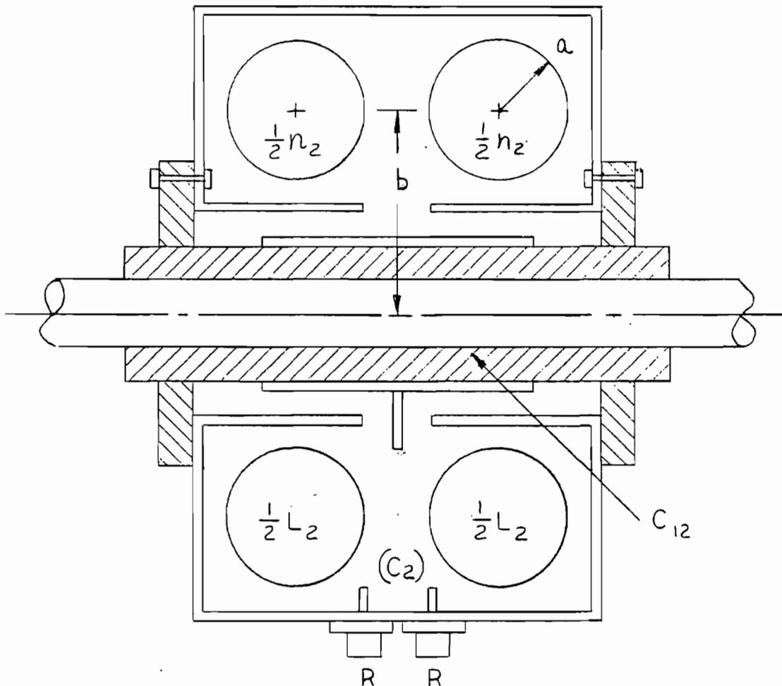
Fig. 7 - Structure details of directional coupler.
