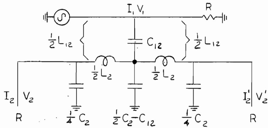
Fig. 6 - Circuit details of directional coupler.
