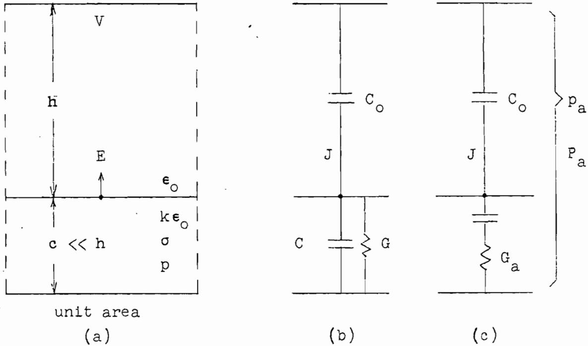
Unit area of ground with plane sheet conductor buried under surface.
