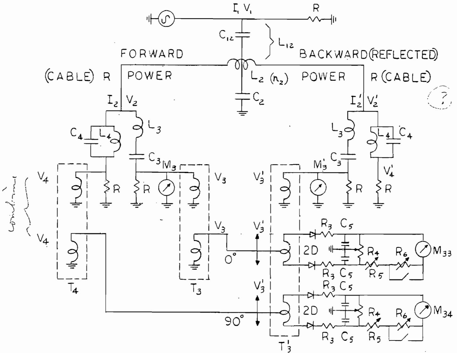
Fig. 4 - Circuit diagram of power and reflection meter.
