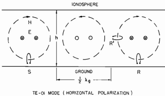
FIGURE 1. Wave propagation in TE-01 mode under ionosphere.
