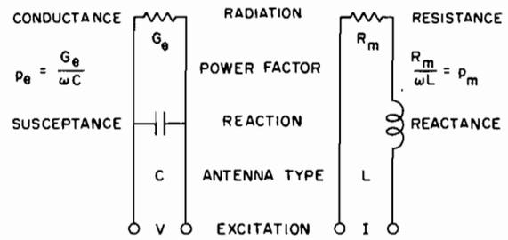
Fig. 2. Radiation power factor of small antenna.
