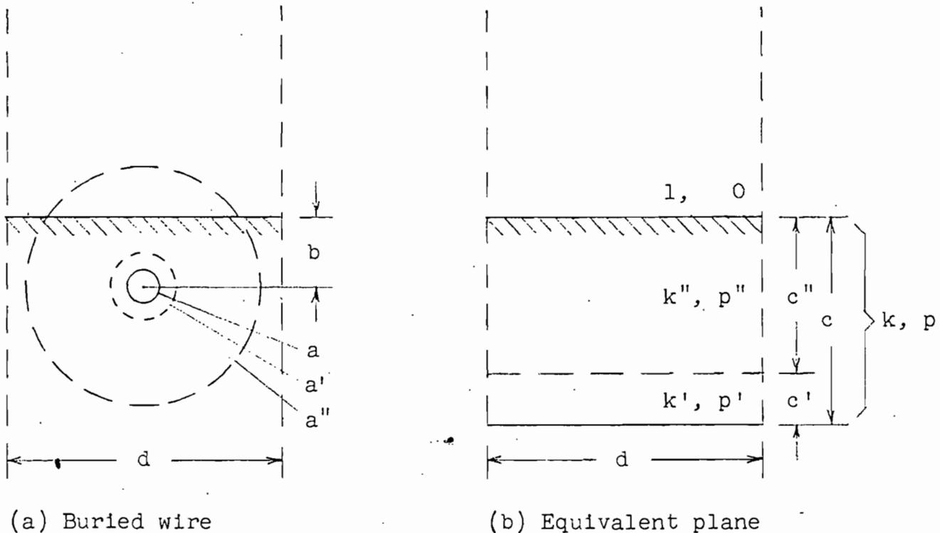
The vertical electric field is associated with a dielectric flux and capacitive current which are terminated at a horizontal grid of parallel wires buried in the ground. In some respects, this grid is equivalent to a horizontal plane conductor buried at a certain depth greater than the depth of the wires. The depth of the equivalent plane will be formulated, also the optimum depth of the wires which minimizes the depth of the equivalent plane.
