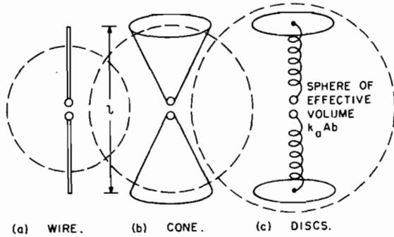
Fig. 6. Effective volume of axial electric dipole.
