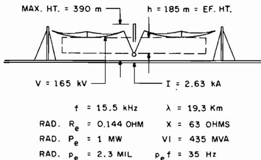
Fig. 18. Large VLF antenna (elevation view).
