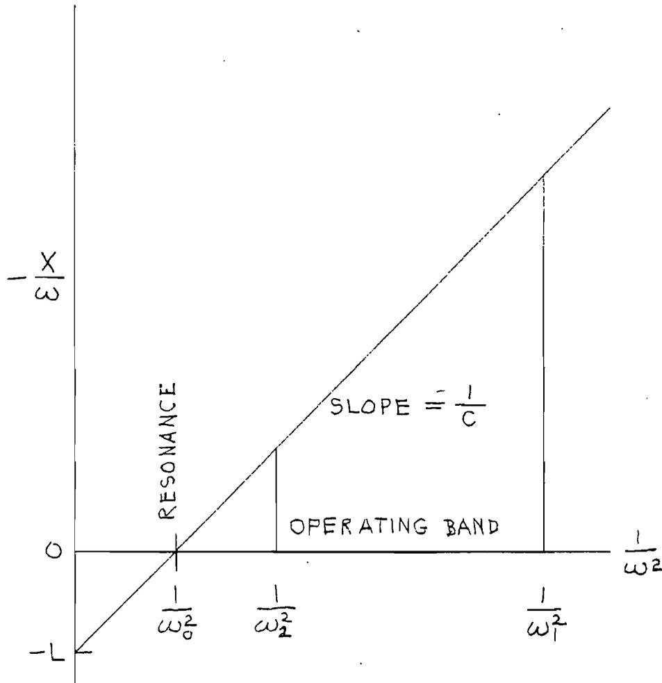
Fig. 8 - Straight-line graph of antenna reactance.
