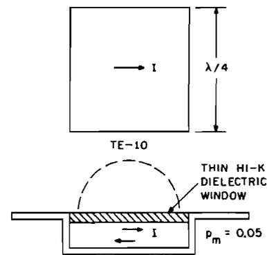
Fig. 11. Flush cavity inductor with dielectric window.
