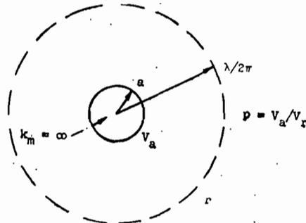
Fig. 8—Spherical inductor in radiansphere.
