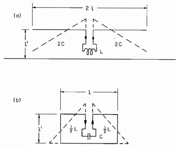
FIGURE 5. Alternative sending antennas on the ground.
