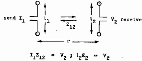
Fig. 1—Definition of mutual impedance between two small electric dipoles.
