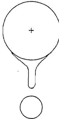
Water drops from an aerial wire are the cause of corona at voltages much too low to cause corona on the clean wire. The direct cause of corona is the excess electric gradient on the lowest side of the falling drop, which is several times that on the clean wire.
