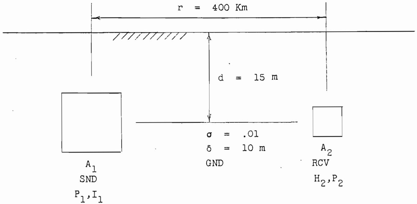
Fig. 1 - Underground antennas for sending and receiving.
