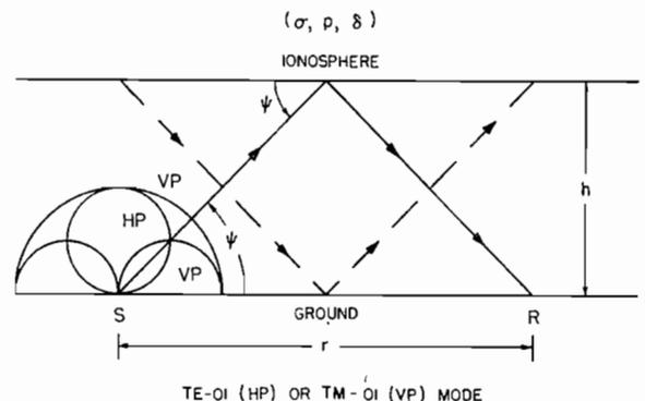
FIGURE 2. Theory of reflection for evaluation of transmission efficiency.
