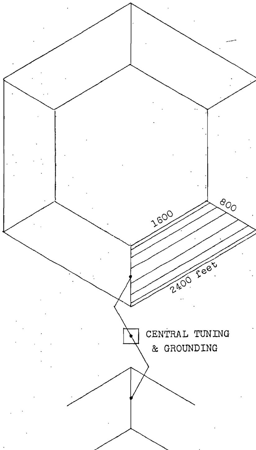
The triatic ring is a pattern of aerial wires which is made of a long triatic with its ends closed to form a polygon (hexagon). This arrangement is proposed to retain the principal benefits of the straight long triatic, while gaining some of the advantages of the six-pointed star and some advantages over either.
