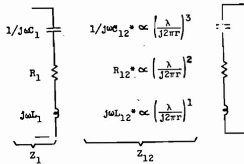
Fig. 5—Network equivalent to two small electric dipoles.
