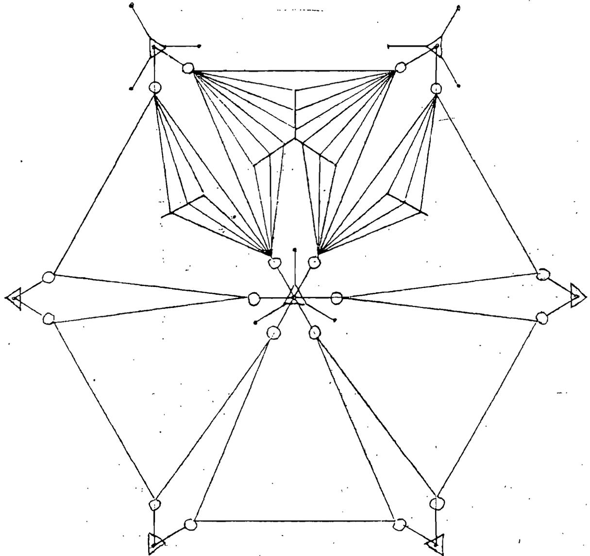
The 6-leaf cross is a form of hexagon pattern for distributing the aerial wires over the flat top. It is proposed to use two such structures to form the independent halves of the entire antenna. Each requires 7 towers, making a total of 14 towers.
