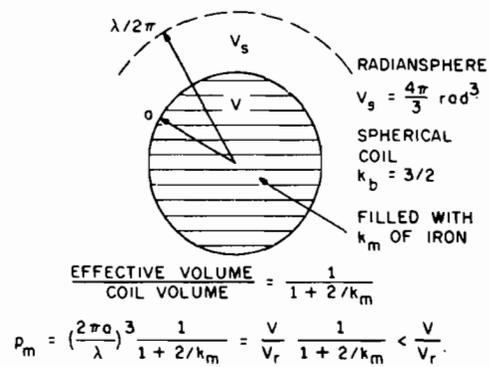
Fig. 5. Spherical coil with magnetic core.
