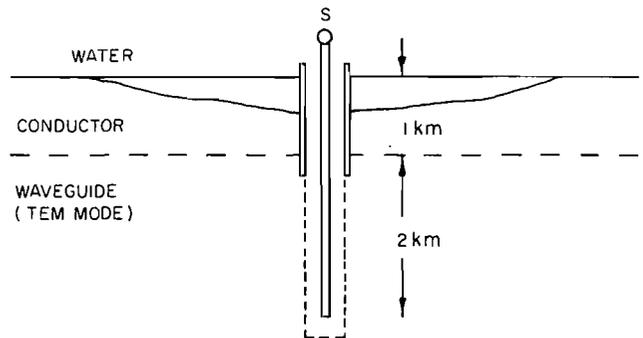
FIGURE 2. Sender antenna in the deep waveguide.
