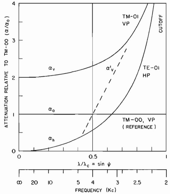
FIGURE 3. Relative attenuation of propagation in modes TM-00, TM-01, and TE-01.
