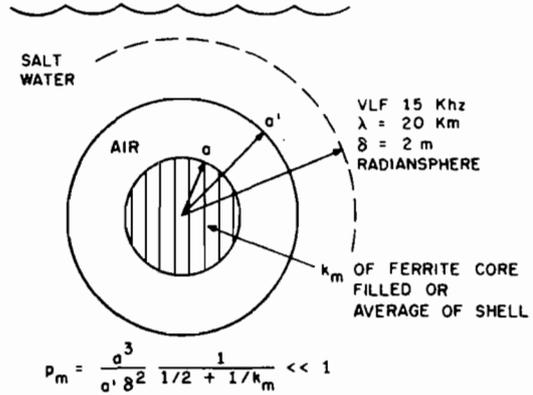
Fig. 15. Inductor in radome submerged in sea water.
