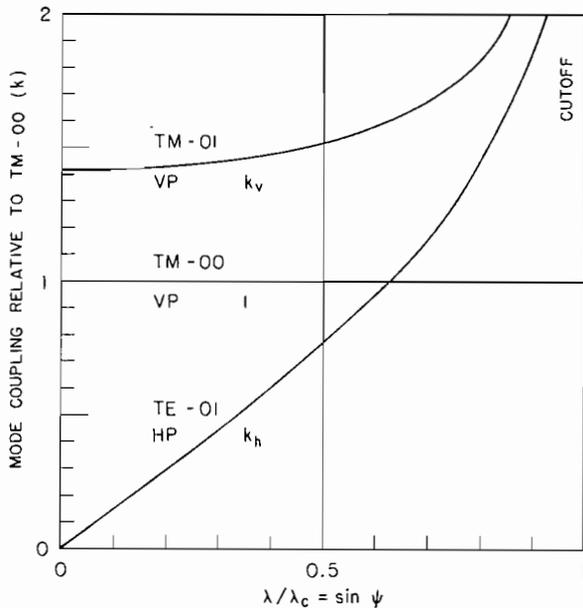
FIGURE 4. Relative mode coupling between loop and modes TM-00, TM-01, and TE-01.
