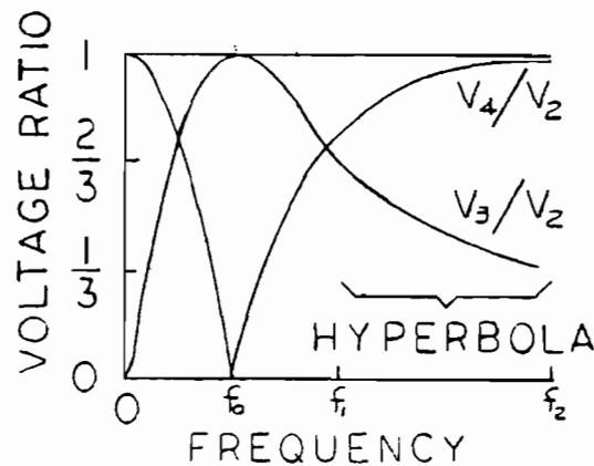
ew Fig. 5 - Voltage ratio inversely proportional to frequency.
